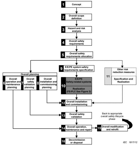
NOTE 1 Activities relating to verification, management of functional safety and functional safety assessment are not shown for reasons of clarity but are relevant to all overall, E/E/PE system and software safety lifecycle phases.
