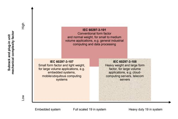
Subrack and plug-in unit system weight factor
