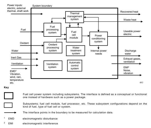
Figure 1 – Fuel cell power system diagram
