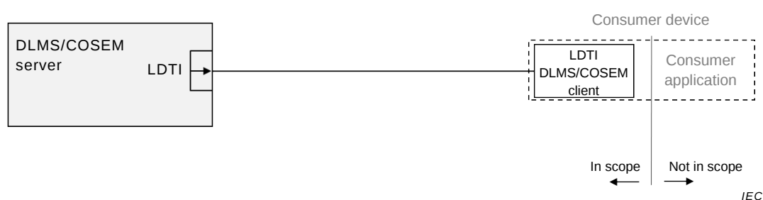
Figure 1 – LDTI DLMS/COSEM client as part of a consumer device
