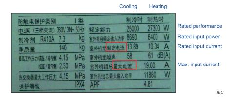
This led to confusion, whether IEC 61000-3-3 or IEC 61000-3-11 is applicable for the evaluation of voltage changes, voltage fluctuations and flicker produced by this equipment.
