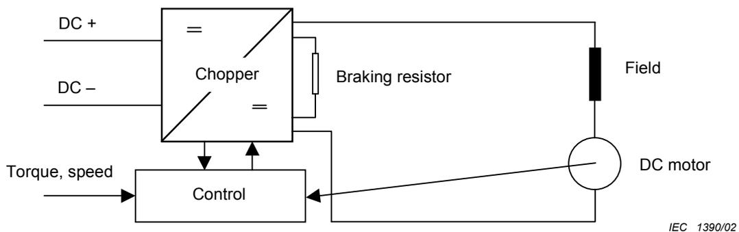
**Figure 1a – Combined system with series d.c. motor**
