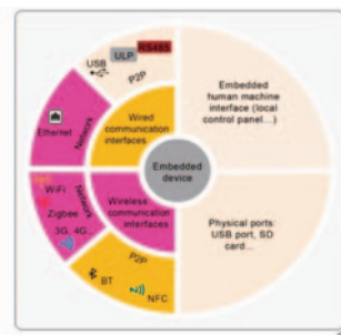
Figure 2 – Example of physical interfaces of an embedded device in an equipment which can be subject to an attack
